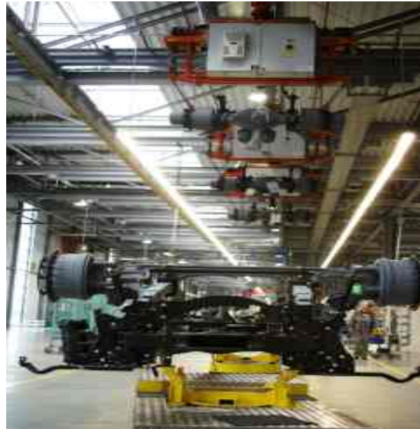
Fig. 2b. An axle carried by a Bluetooth controlled motion system is mounted in a vehicle frame carried by an automatic guided transportation system controlled via Wi-Fi.
