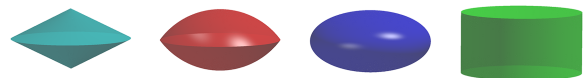
FIG. 9. Oblate solids of revolution with an aspect ratio of \nu = 1/2 . From left to right a double cone, a lens, an ellipsoid, and a cylinder are displayed. All shapes to the left of a given geometry are strict subsets of their right neighbors. The lens and the ellipsoid approach in the limit \nu \rightarrow 1 a sphere. While a lens does only exist with aspect ratios \nu \leq 1 , prolate analogs of double cones, ellipsoids, and cylinders with \nu > 1 exist.
