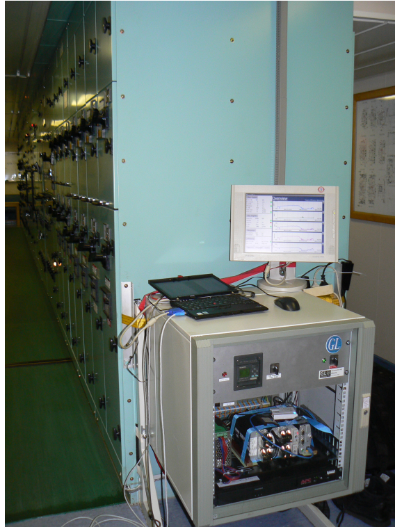
Figure 5.2. EEMT test installation in the engine control room of the postpanmax container vessel.
