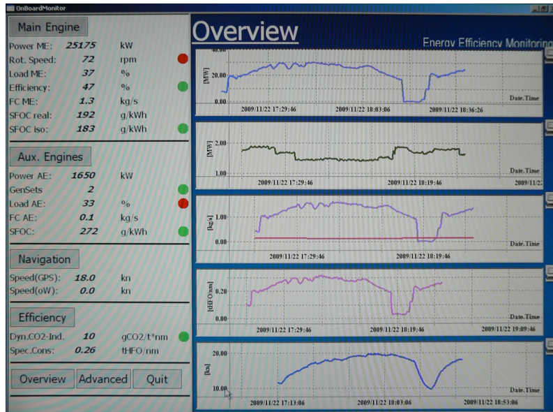
Figure 5.3. Picture of the EEMT screen during sea passage, red traffic lights indicating high ship resistance and low auxiliary engine load.
