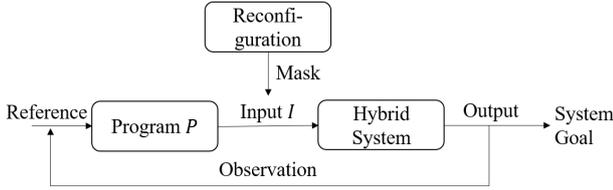
Figure 1: Reconfiguration masks some inputs of the hybrid system such that a control program can reach the system goal.
