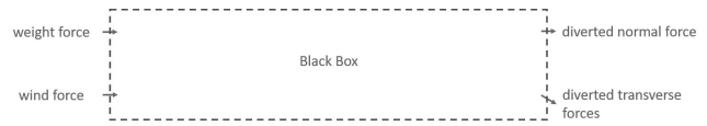
Figure 2: Bridge as a Black Box - Here the overall function of bear (dynamic) force is not decomposed. The function has an in-degree of 2 (weight force and wind force) and an out-degree of 2 (diverted normal force and diverted transverse forces)
