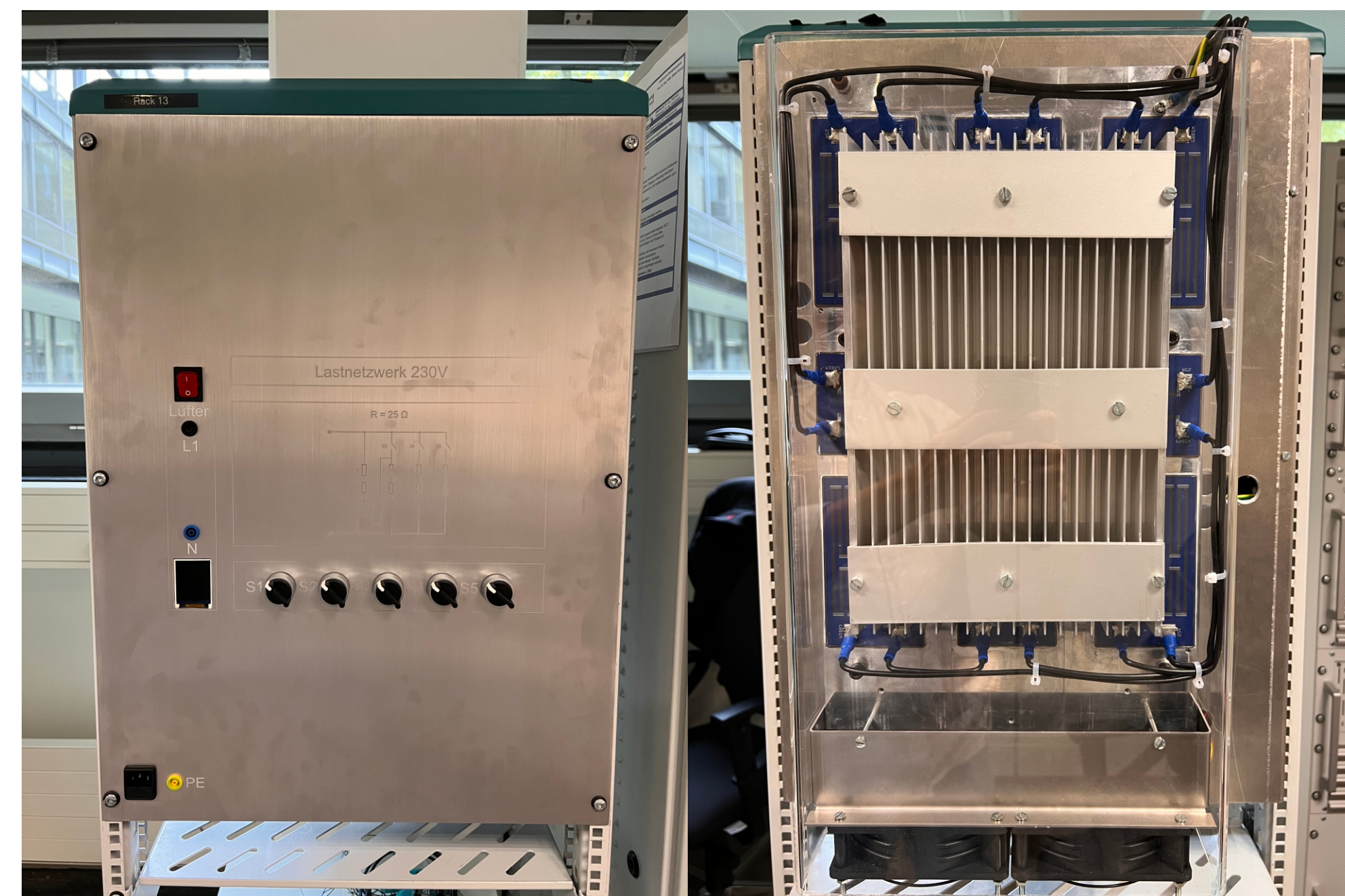
Figure 2 Non-linear load test bench, frontside left, backside right.
