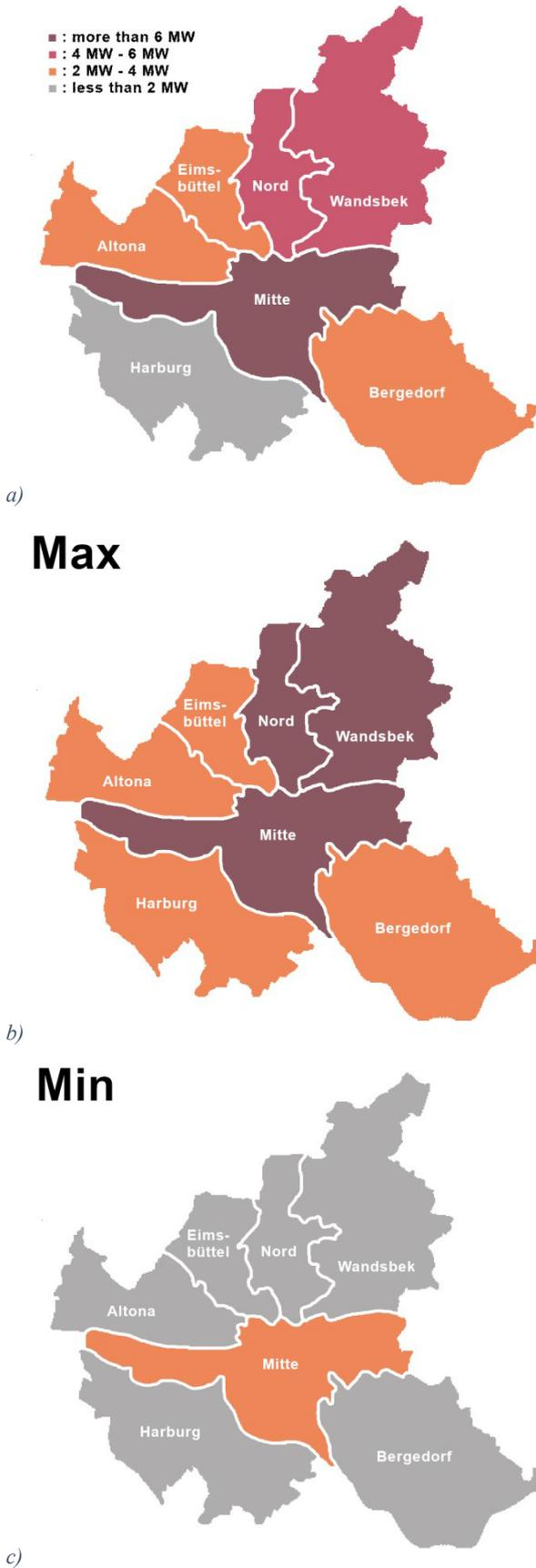
FIGURE 5: PROJECTION OF THE TOTAL PEAK DEMAND FOR THE HAMBURG BOROUGHS BY ELECTRIC TRUCK CHARGING IN 2050 (A - AVERAGE, B - MAXIMAL, C - MINIMAL SCENARIOS).
