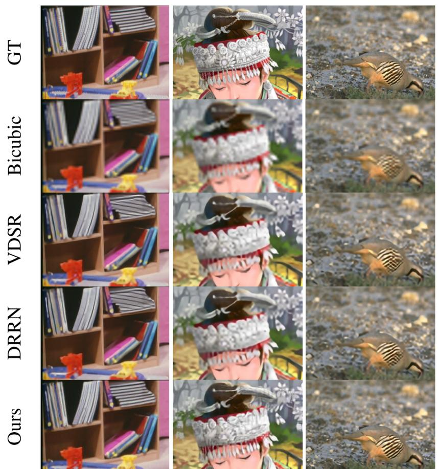
The ground truth (GT) and examples of non-blind super-resolution for a scale of  $\times 4$  with bicubic interpolation, very deep super resolution (VDSR) network, deep recursive residual network (DRRN) and our method.
