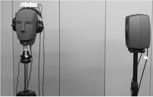
Fig. 4. Measurement setup overview. Dummy head (left) wearing the ANC headphone and external loudspeaker (right) used to generate the auxiliary impulse responses.
