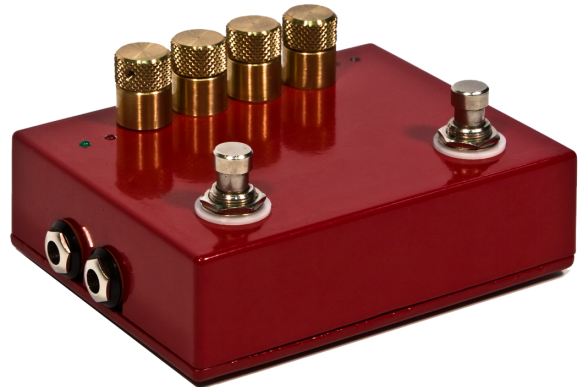
Figure 1: Picture of the GEB1. The four knobs in the rear are the potentiometers and the encoder, ahead the two foot switches.
